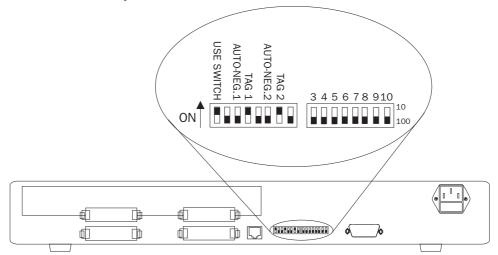
**Note:** The DIP switches described below function only when the USE SWITCH switch is in the ON position.
